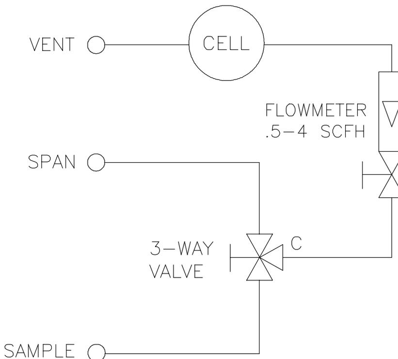
*Figure 3-3: Piping Diagram
