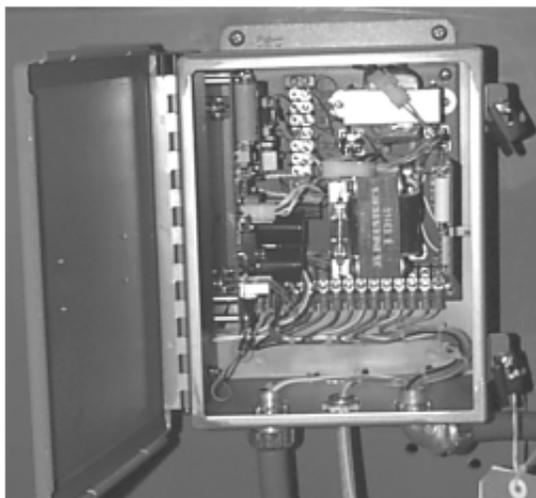
Source Power Supply and optional Temperature Controller PCB
