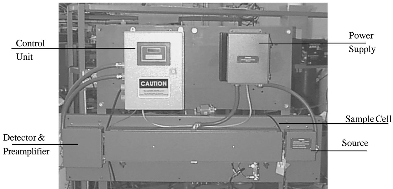
Model 6000B Photometric Analyzer with D2 Lamp
