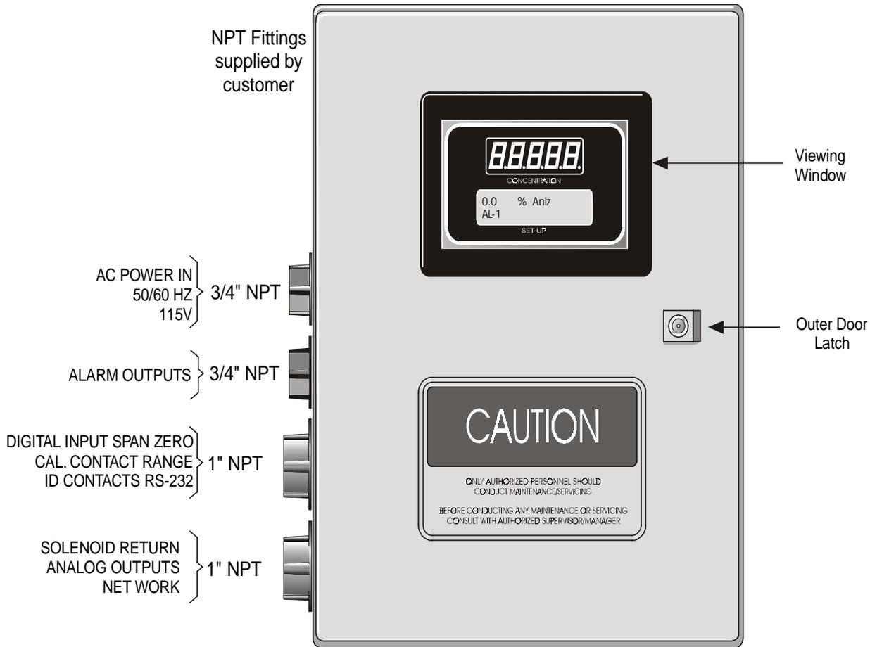
Figure 2-1: Front Panel of the Model 6000B Control Unit
