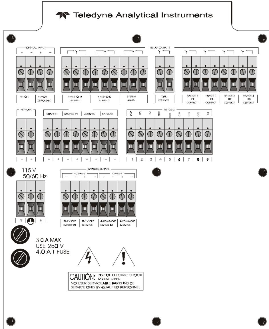
Figure 1-2: Model 6000B Rear Panel
