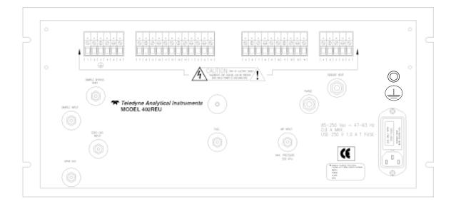
Figure 3-1: Rear Panel of Model 402R-EU With Gas Connections
