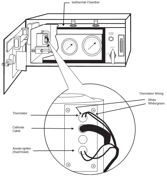
Figure 5-2: Identification and Location of Thermistor and Wires
