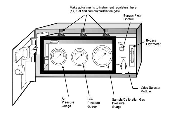
Figure 4-2: Setting the Air, Fuel and Sample Pressure
