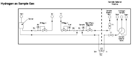
Figure 1-1A: Schematic Flow Diagram With Gas Selector Panel
