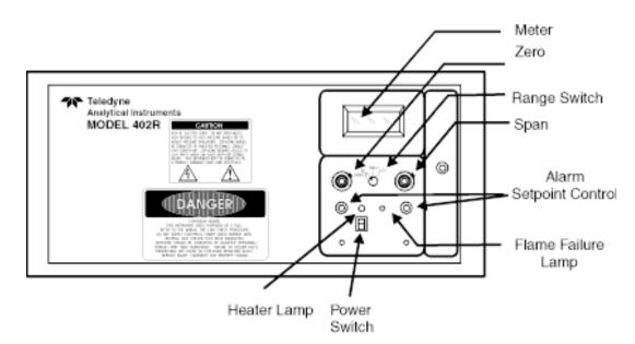
Figure 4-1: Front Panel of Model 402R-EU Total Hydrocarbon Analyzer
