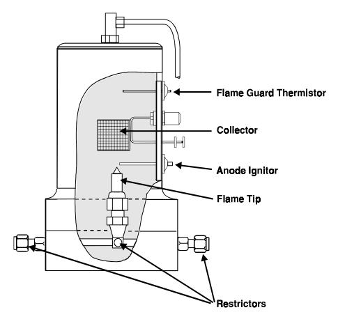
Figure 1-2: Flame Ionization Cell
