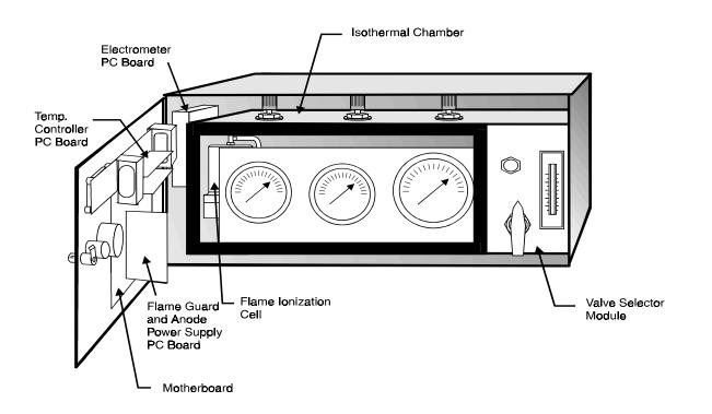
Figure 2-1: View Inside 402R-EU Cabinet (with internal door cover removed)
