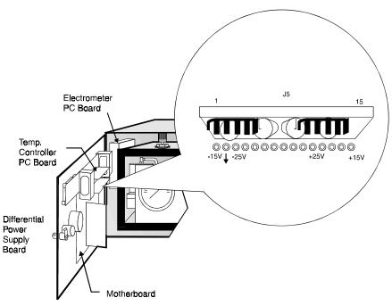
Figure 5-1: Checking the Differential Power Supply
