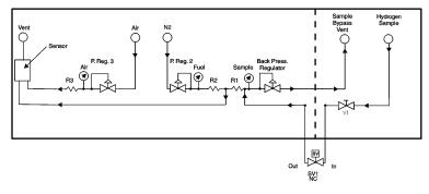
Figure 1-1B: Schematic Flow Diagram Without Gas Selector Panel
