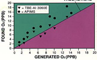
Plot shows excellent agreement between the calculated oxygen concentration vs. experimental values obtained using the most sensitive range of the analyzer (0-50 ppb O<sub>2</sub> full scale).
