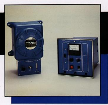
The Micro-Fuel Cell produces an output that is linear from 0 to 100%. That means you can use ambient air (209,500 ppm  $O_2$ ) for calibration. This eliminates the need for special ppm  $O_2$  span gases. Or, if a faster calibration is required, a certified ppm  $O_2$  span gas can be used to calibrate the Model 317R.
